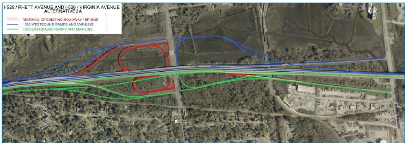
Figure 1.6: Proposed interchange configuration at North Rhett and Virginia Avenues in North Charleston
