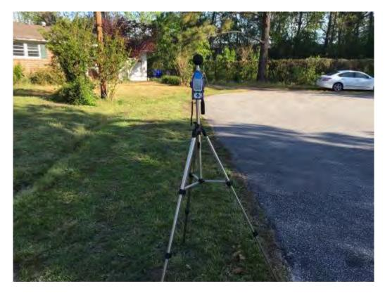
Figure A.53. I-526 WEST – Ambient Noise Monitoring Setup 32, Receptor 32a
