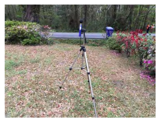
Figure A.2. I-526 WEST – Ambient Noise Monitoring Setup 1, Receptor 1a
