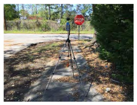
Figure A.46. I-526 WEST – Ambient Noise Monitoring Setup 28, Receptor 28
