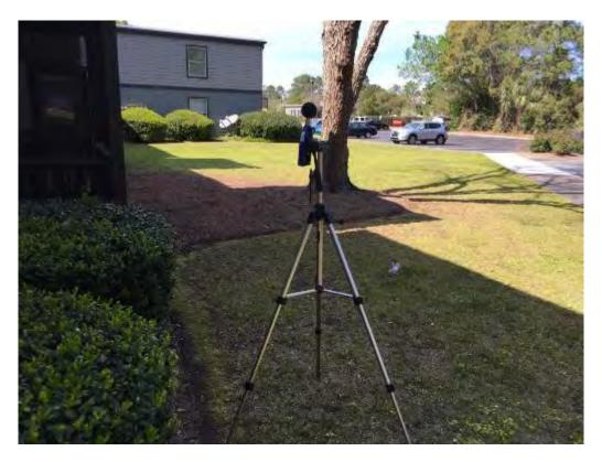
Figure A.17. I-526 WEST – Ambient Noise Monitoring Setup 6B, Receptor 6B-a
