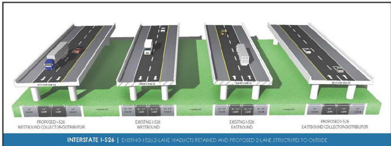
Figure 6-2. Typical Section of Improvements and New Viaduct Over Filbin Creek
