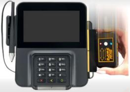
Following these steps ensures that your Skim Swipe will detect skimmers on both sides of the card slot especially in newer model card swipers
