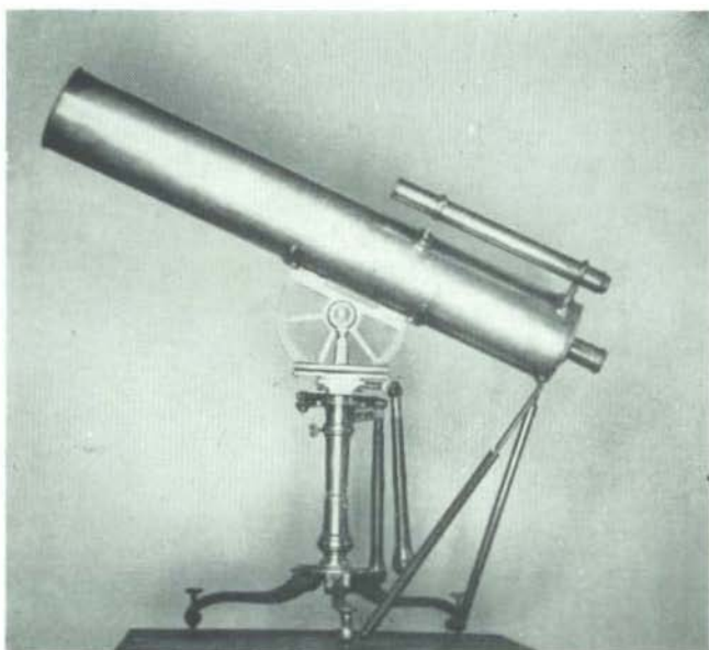
GREGORIAN REFLECTOR OF 4-INCH APERTURE AND 24-INCH FOCAL LENGTH USED IN THE OBSERVATION OF THE TRANSIT OF VENUS, JUNE 3, 1769, NOW IN LADD OBSERVATORY, BROWN UNIVERSITY. Photograph by C. H. Smiley.
