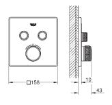
Grohtherm SmartControl Thermostat for concealed installation with
