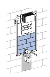
Geberit Kombifix installation elements are exclusively suitable for solid construction. They must be fastened in front of or inside a solid wall and then subsequently brick lined.
