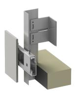
Tiles with a thickness of 14 mm can be fitted invisible on the back with metal clips and special dowels. For this purpose, each panel has on the top row of clips adjusting screws and a fixed point fastening (screw or clip), with the result that it can be aligned and no displacement occurs.
