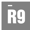
Low Friction High slip risk Slip Angle 6-10° Suited to indoor domestic applications
