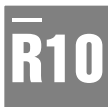
Medium Friction Moderate slip risk Slip Angle 10-19° Suited to indoor commercial applications
