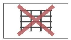
Novowood products are coating materials that, despite their mechanical strength characteristics, must always be laid on a supporting subconstruction framework of a suitable size.
