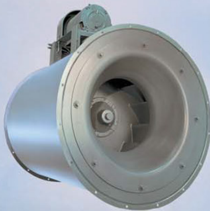
Belt Drive Wheel Sizes: 10.5"-49" Direct Drive Wheel Sizes: 10.5"-36.5" CFM Range: 435-67,407 Static Pressure: Up to 8.5" WG
