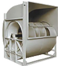
Wheel Sizes: 5"-12.5" CFM Range: 100-3,350 Static Pressure: Up to 2.75" WG
