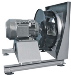
Wheel Sizes SWSI: 12.25"-24.5" and 27"-49" CFM Range Wheel Sizes (12.25"-24.5"): 686-13,140 CFM Range Wheel Sizes (27"-49"): 2,514-74,520 Wheel Sizes DWDI: 12.25"-24.5" CFM Range DWDI: 1,548-34,877 Static Pressure: SWSI Only (27"-49"): Up to 20" WG SWSI/DWDI Only (12.25"-24.5"): Up to 13.5" WG
