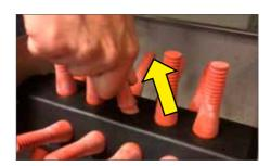
2 Take a screwdriver and push the fingers with this screwdriver in the drum. As shown in picture beside.
