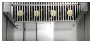
Fans provide 'Laminar Airflow'
