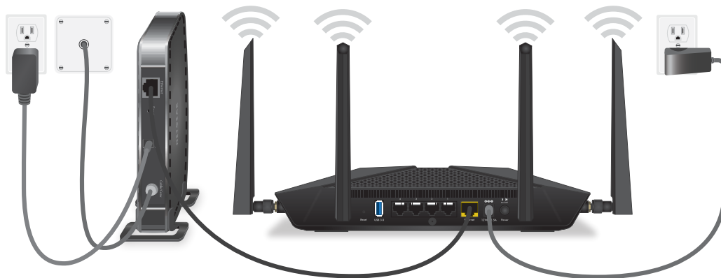
Figure 7. Cable your router
