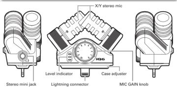
X/Y stereo mic: This is an X/Y format stereo mic. You can set the recording angle to 90° or 120° by turning the individual mics. (See "Adjusting the stereo width.")
