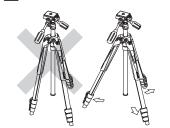
To prevent accidental falls or tripod tipping over, making sure all levers, knobs and handles on the tripod are securely tightened.
