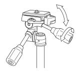
Loosen the vertical til handle, and the level can be adjusted.
