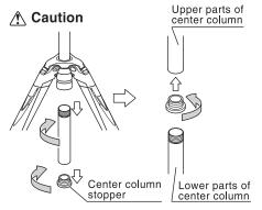
Turn the lower part of the center column in the direction of the arrow. (counter clockwise) Attach the center column weight hook to the bottom of the upper center column to prevent the center column from falling out of the body.
