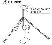
Insert the center column from the lower side of main body, and tighten the center column lock.
