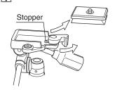
Remove the quick release shoe by turning the shoe locking lever to release.
