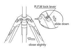
Close the leg slightly and slide the R.F.M lock lever down.
