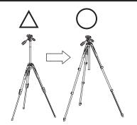
For best results and to avoid unnecessary camera vibrations, try to keep the center column height to a minimum if possible.
