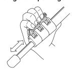
Flip the leg lock lever up to extend or shorten the section to the desired length.
