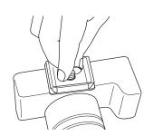
Insert the camera mounting screw of the shoe in the place of the tripod mounting screw of your camera. Turn the camera mounting screw knob and fix firmly.
