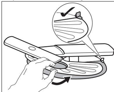
7. Reassemble the filters (B) and (C).
