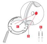
2. To achieve the correct smoke alarm positioning, you can direct your smoke alarm with the aid of the direction arrow (C) on the mounting plate. The arrow indicates the final position of the smoke alarm: square edge for Kupu and head for Lento.
