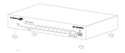
2. Rack-mount the switch: You can mount the switch in any standard size, 19-inch (about 48 cm) wide rack with 1 Rack Unit (1U) of space, which is 1.75 inches (4.45 cm) high. A pair of extension brackets and screws are needed to adapt the switch to the rack size.
