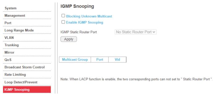
NOTE: When "Enable IGMP Snooping" is selected, IGMP Static Router Port can be selected using the drop down menu.
