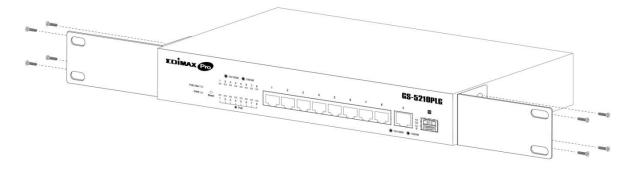
Secure the switch on the equipment rack with the screws provided.
