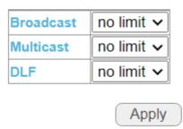
Select a limit in the drop down menus behind the storm control features and click "Apply" to apply the settings.
