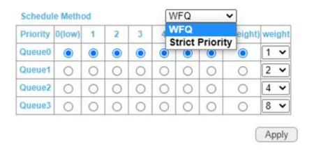
If QoS type is set to 802.1p, the priority is based on the incoming PCP field of the traffic. The current queue for each PCP is configured as below.
