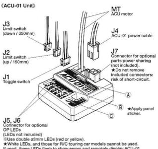
If used, these LEDs flash to show errors and remotely display ACU-01
