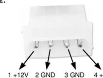
For using the EX-11494-2 you must connect the card with the PC power supply. It must be connected only one power connector J1 **OR** J2! Please make sure you connect the plug in the right direction.
