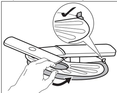
7. Reassemble the filters (B) and (C).
