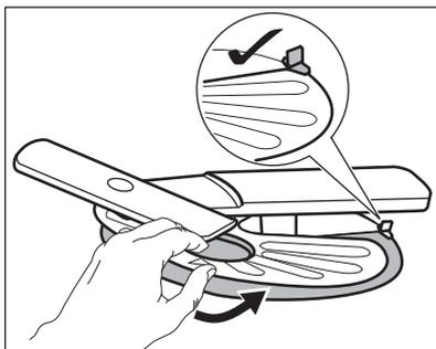
7. Reassemble the filters (B) and (C).
