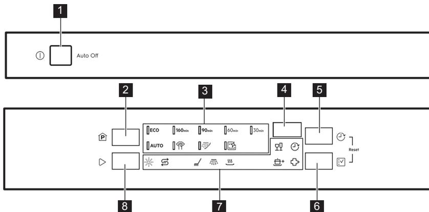
**1** On/off button**2** Program button**3** Programme indicators**4** Display**5** Delay button**6** Option button**7** Indicators**8** Start button**4.1 Indicators**
