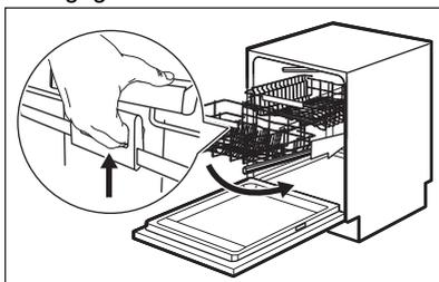
Once the basket is unlocked, push the rack down. The mechanism
