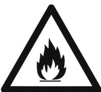
The cooling circuit in this appliance contains the refrigerant isobutane (R600a), a natural gas
