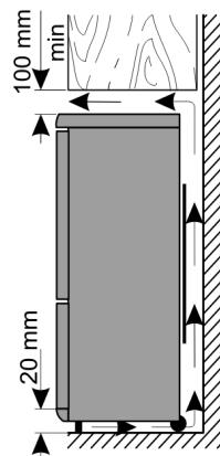
The heated air around the rear of the unit must be able to circulate freely.
