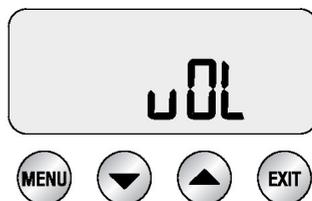
Use this function to set Duration or Volume to control the espresso output.
