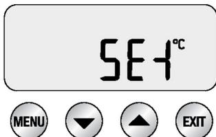
Temperature Unit will be displayed on the LCD screen as SEt. Press MENU to Select.
