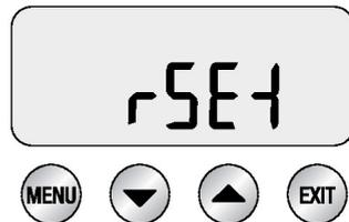
The machine will then prompt you to set the water hardness. Select your water hardness using the UP & DOWN arrows & press MENU to confirm or press EXIT to return to STANDBY mode.
