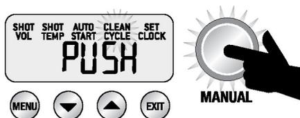
The CLEAN CYCLE icon will flash and the machine will start to countdown from 370 seconds.
