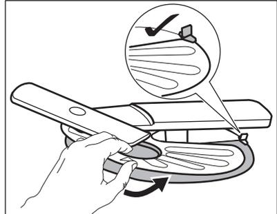
7. Reassemble the filters (B) and (C).
