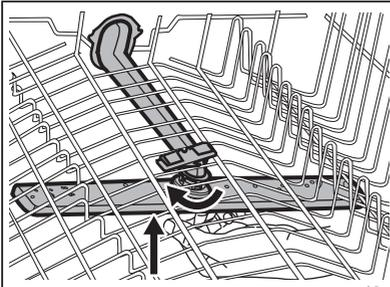
3. Wash the spray arm under running water. Use a thin pointed tool, e.g. toothpick, to remove particles of soil from the holes.
