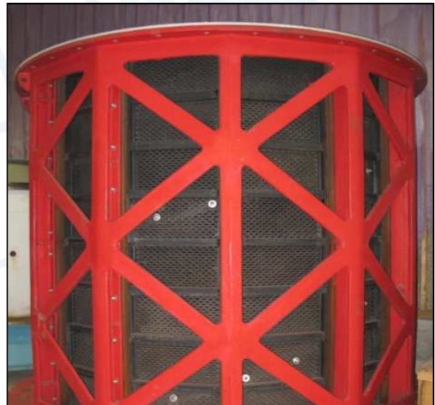
Discharge Trommel Painted
