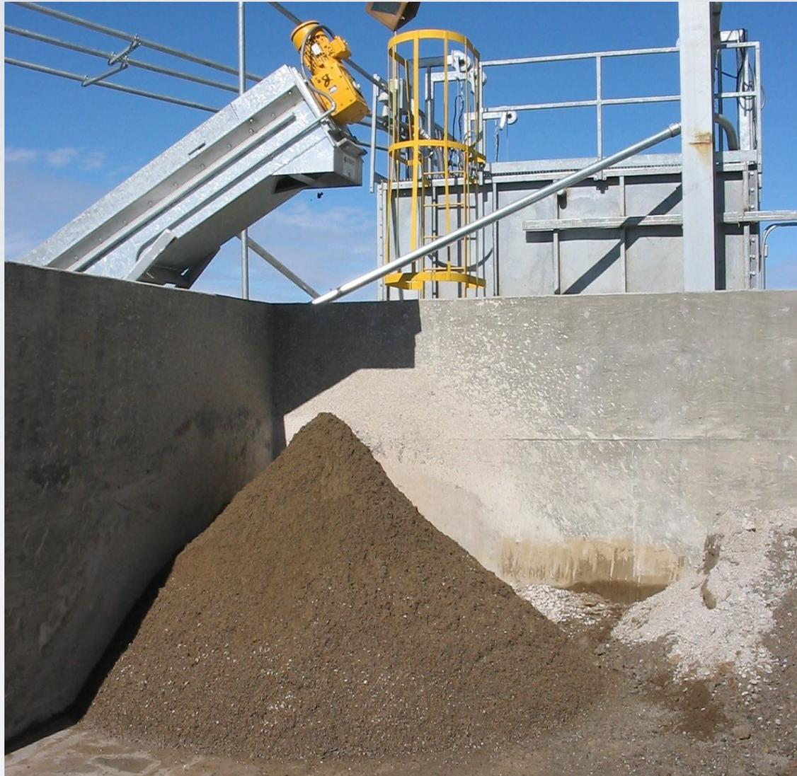
DISCHARGE OF CLEANED SAND AND AGGREGATE
