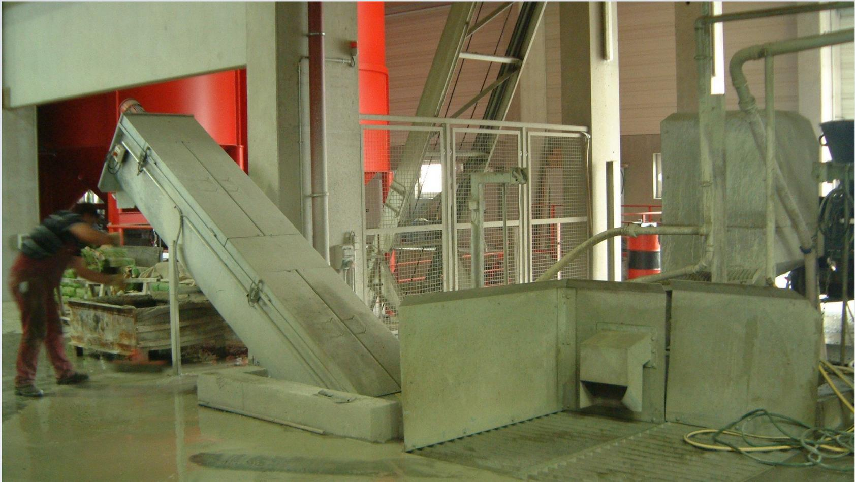
**BIBKO PRECAST CONCRETE RECLAIMER AND WASHOUT SYSTEM**
