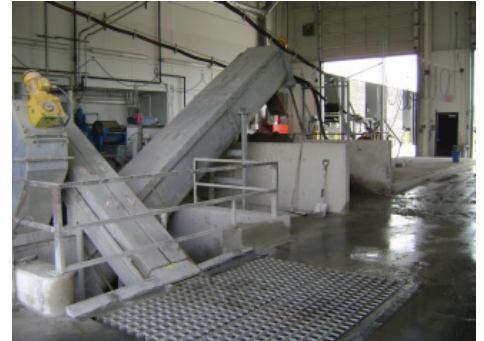
PDC Pump Discharge Conveyor charging BIBKO® 1000
