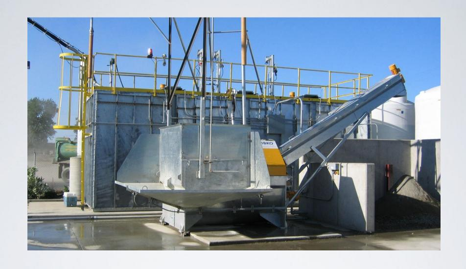
ZERO DISCHARGE CONCRETE RECLAIMING
