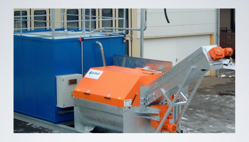
PORTABLE BIBKO 2000 CONCRETE RECLAIMER WITH 5,000 GALLON SLURRY TANK
