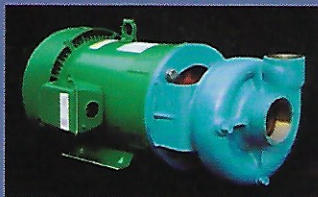
CENTRIFUGAL PUMPS: PLANT SUPPLY PUMPS 10 or 7.5 hp, 230-460 V, 3-phase, 3500 rpm.
