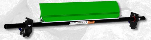
The Eraser RPQ system uses the same simple and effective spring tensioning unit as the Eraser PQ, with a 7" tall polyurethane blade, giving you more wear life and allowing for installation on systems with a larger diameter head pulley.
