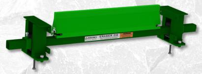
The Eraser DS is an economical version of our XTC cleaner, with a .19" thick, 2"x 2" powder-coated tube stock steel mainframe for strength and durability. The DS uses the same polyurethane blade as the XTC.
