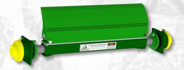
The Super Eraser is a Mine Duty cleaner. It has a .25'' thick, 3.5'' x 3.5'' box steel mainframe and a massive 12" polyurethane blade. It will handle anything you throw at it. If you're dealing with high speed, high tonnage belts, the Super Eraser was built specifically for you.
