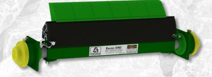
The Eraser SHD utilizes the Super Eraser mainframe and Safe Torque tensioners paired with an 11.25" tall replaceable tip blade. A mine duty design, this heavy-duty system allows for only the 6" blade tip sections to be replaced when they become worn, rather than the entire blade length.
