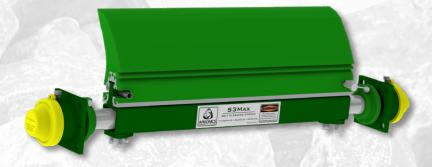
The S3Max is an intermediate system between the Eraser and the Super Eraser that features a 10" tall polyurethane blade. It is ideally suited for more aggressive applications where a larger blade is required, or those systems with a larger head pulley.
