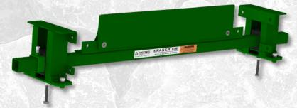
The Eraser DS tungsten system is urethane-free for use with high-temperature materials. It uses the same .19" thick, 2"x 2" powder-coated tube stock steel mainframe as the DS system. It also utilizes the same tungsten carbide blades as the XTC.
