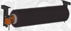
The Brush Cleaner is a completely contained system, which utilizes a Van der Graaf drum motor. This motor is an enclosed unit with all motorized parts inside the roller, making it the choice for the most challenging environments. The compact, low-profile design operates at 96% efficiency and is virtually maintenance-free. It is ideal for use on chevron or cleated belts.
