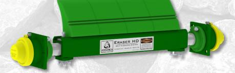
The Eraser HD is designed to withstand heavy vibration. This system has a reinforced mainframe and a heavy-duty channel attachment design. It utilizes a series of 6'' wide  $\times$  7'' tall polyurethane blade segments that conform to crowned head pulleys.
