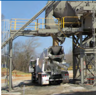
Mixer Maintenance Platform and Dump Cone
