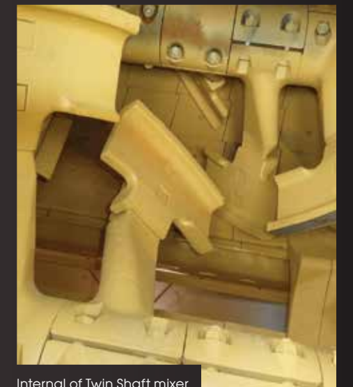
Internal of Twin Shaft mixer
