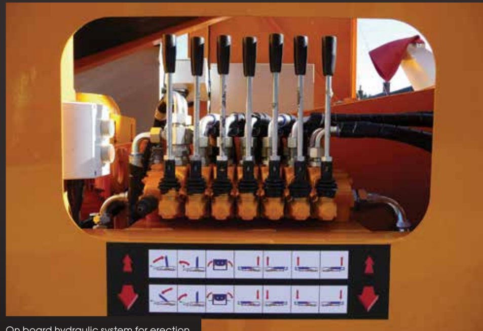
On board hydraulic system for erection
