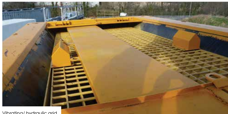
Vibrating/ hydraulic grid
