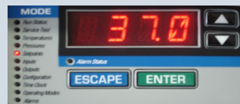
diagnostic Display & Control module Scrolling Marque
