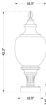
Full Acorn, "5P" Fitter, Pier Base (450PB-A850-5P)
