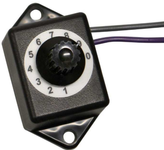
Fixed Dimming Resistor Board (FDRB)
