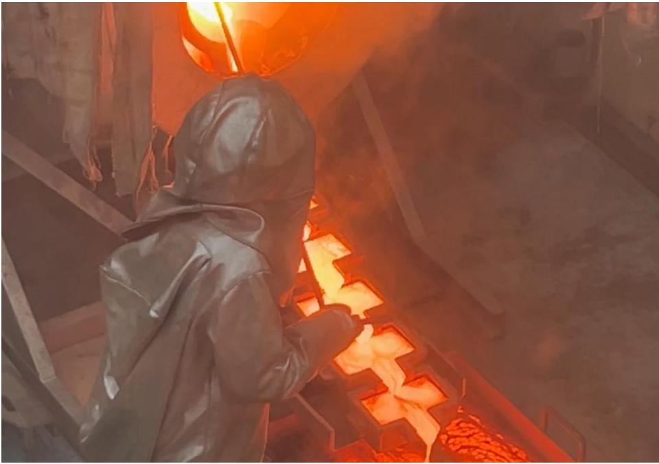
Figure 7. Gold Room smelting process to produce doré bullion
