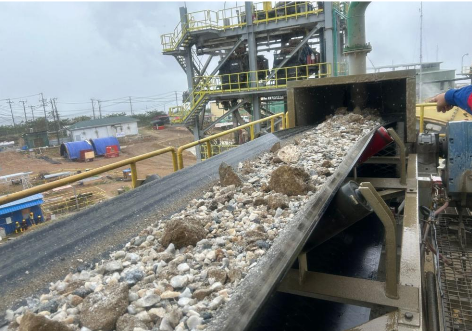
Figure 2. Conveyor to Transfer Crushed Ore to Sag & Ball Mill
