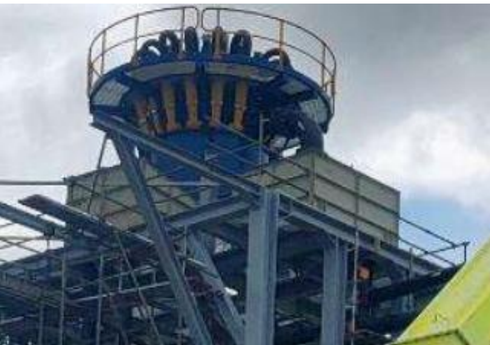
Figure 4. Cyclone separates coarse (+75 µm) and fine (–75 µm) ore fractions
