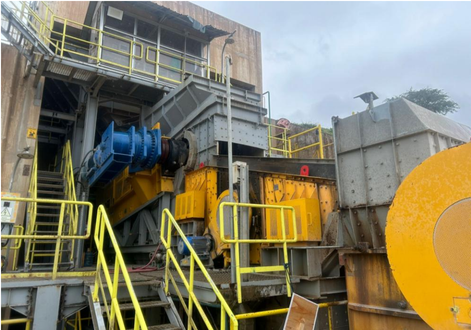
Figure 1. Jaw Crusher to Crush Mined Ore
