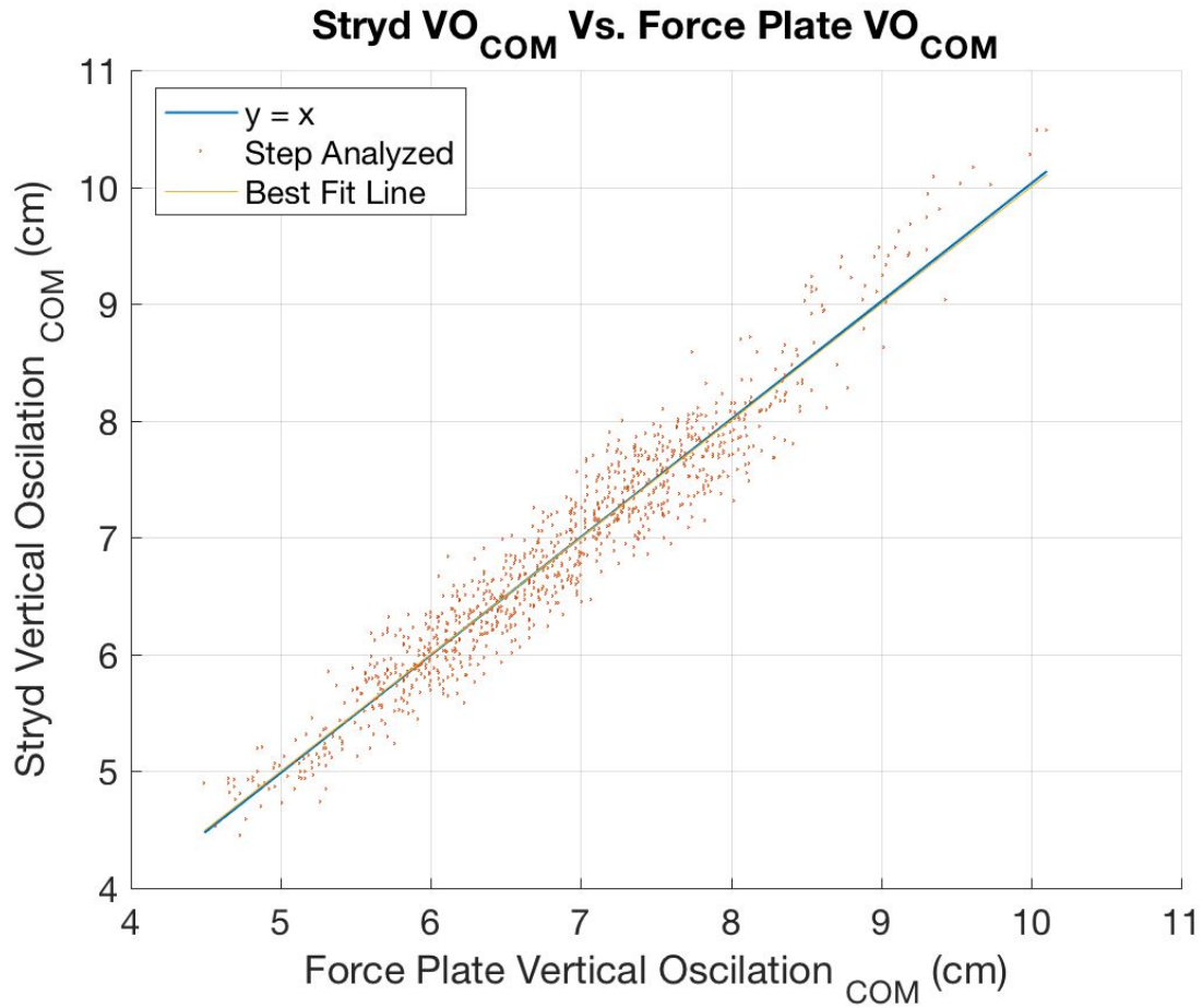
FIGURE 8. Stryd’s vertical oscillation (centimeters) vs force plate vertical oscillation (centimeters) comparison. Average magnitude error: 3.18%
