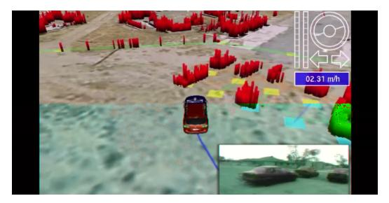
Again, the car is using A\* to find the optimal path into this parking lot, and then back in and back out again. The planning run for each of these A\* runs is less than 10 msec. The car was able to competently do this, even though in advance it had no clue where the obstacles were and where the parking spot was.
