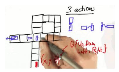
The world looks a bit different now with representation of the streets that are navigable and with a loop on the right side. Remember that the state-space now is 3-dimensional, since each cell in the 2D grid now has an additional dimension associated with the robot's orientation.
