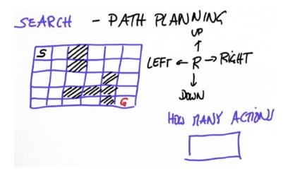
The first step towards writing this program is to name the grid cells. Across the top, name the columns zero to five, and along the side you can name the rows zero to four. Think about each grid cell as a data point, called a node and the goal point is called the goal node.
