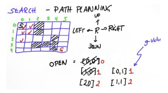
The next lowest g-value is the cell [0,1], but since the surrounding cells, [0,0] and [1,1], are already checked it cannot be expanded any further. The process of expanding the cells, starting with the one with the lowest g-value, should yield the same result you found as the number of moves it takes to get from the start to the goal -- 11.
