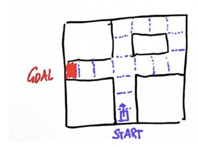
Assume that for each time step you can make one of two actions -- either move forward or turn the vehicle. Each move costs exactly one unit.
