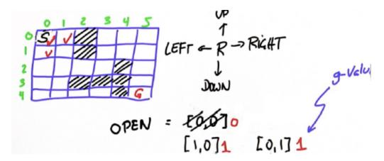
Continue to expand further. Always expand the cell with the smallest g-value, but since the two above are equivalent, it doesn't make a difference which one you expand first. In the image below, the first cell is expanded to include the unchecked cells, [2,0] and [1,1], each with a g-value of two.
