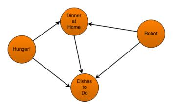
In the network above, each node represents a variable, and arrows from different nodes represent conditional independence assumptions related to the variables. More on this below. For brevity, we will be referring to these variables as
