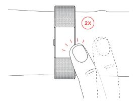
Charge 2 doesn't respond to swipes. You must use the button or firmly and quickly tap the screen.
