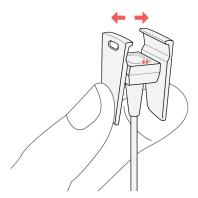
3. Make sure the button on your tracker is aligned with the button opening on the charging cable. You'll know the connection is secure when the tracker vibrates and you see a battery icon on your tracker's display. Your Charge 2 will begin charging.
