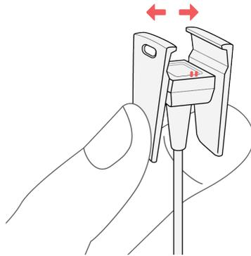
3. Make sure the button on your tracker is aligned with the button opening on the charging cable. You'll know the connection is secure when the tracker vibrates and you see a battery icon on your tracker's display. The battery icon disappears after three seconds.
