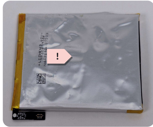
Swelling or electrolyte leakage
