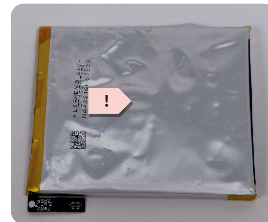
Swelling or electrolyte leakage
