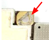
Incorrect: Washer broken
