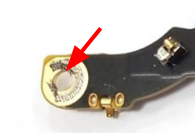
Incorrect: Washer broken
