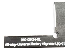
Universal Battery Alignment Jig G940-00424-01
