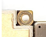
Correct: Washer in good condition
