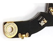
Correct: Washer in good condition
