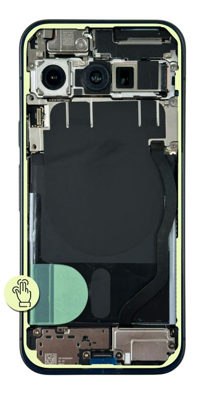
closure Top Speaker Logic Board Mic3 flex Rear Camera mmWave Module Front Camera Display Vibrator Chin Board Bottom Speaker Battery **BG sub**
