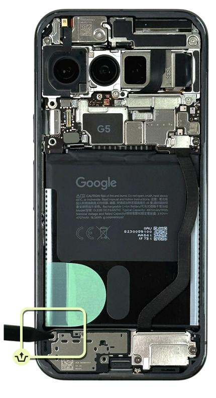
olay BG sub Front camera mmWave Module Mic3 flex Battery Rear Camera Logic board Top Speaker **Bottom speaker** Chin board Vibrator Enclosure
