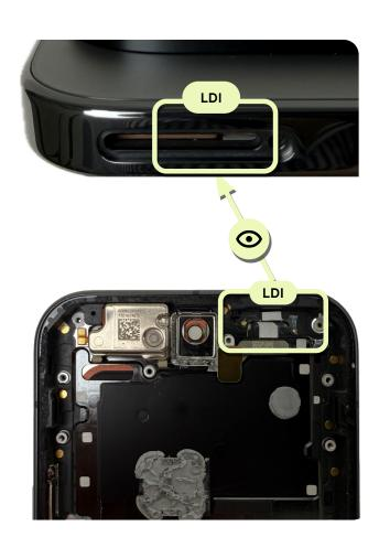
The SIM card tray slot on the enclosure is visible without disassembly of the device.
