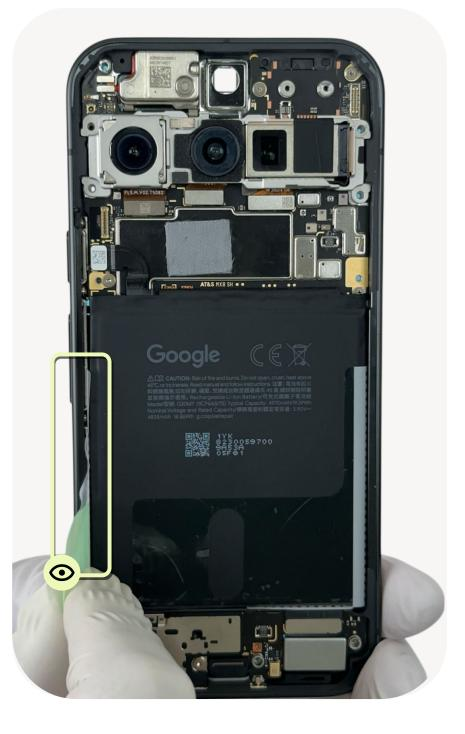
ay BG sub Front camera mmWave Module Mic3 flex **Battery** Rear Camera Logic board Top Speaker Bottom speaker Chin board Vibrator Enclosure
