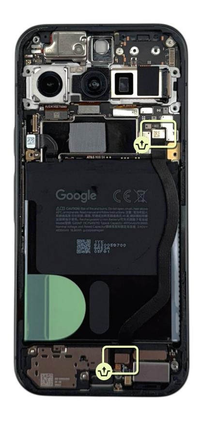
lay BG sub Front camera mmWave Module Mic3 flex **Battery** Rear Camera Logic board Top Speaker Bottom speaker Chin board Vibrator Enclosure
