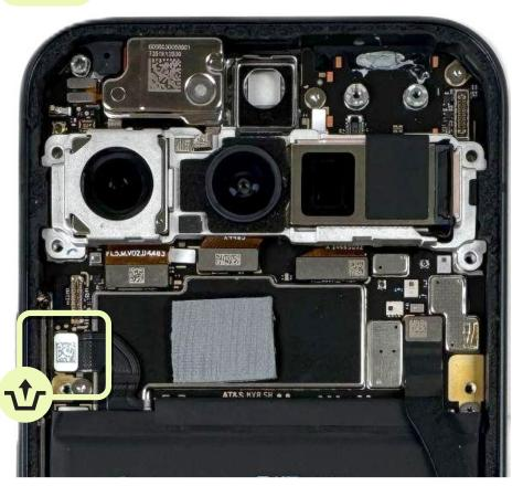
splay BG sub Front camera mmWave Module Mic3 flex **Battery** Rear Camera Logic board Top Speaker Bottom speaker Chin board Vibrator Enclosure
