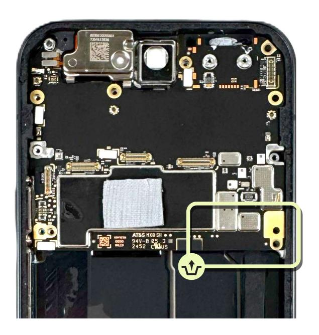
olay BG sub Front camera mmWave Module Mic3 flex Battery Rear Camera **Logic board** Top Speaker Bottom speaker Chin board Vibrator Enclosure
