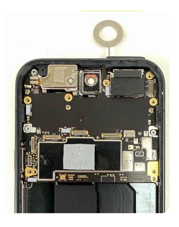
lay BG sub Front camera mmWave Module Mic3 flex Battery Rear Camera **Logic board** Top Speaker Bottom speaker Chin board Vibrator Enclosure
