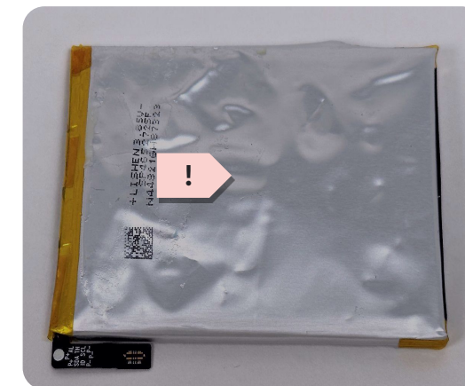
Swelling or electrolyte leakage
