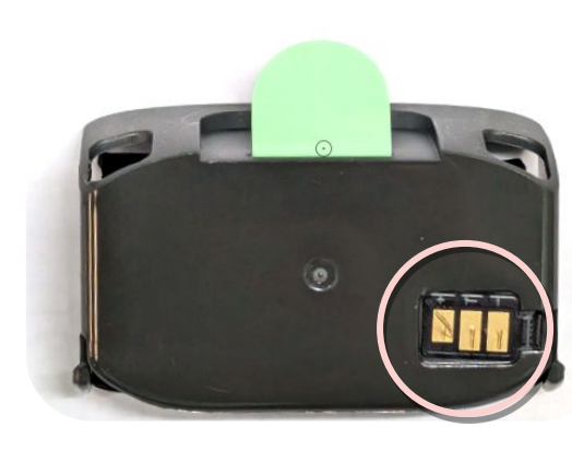
The battery contact pad is dirty or oxidized
