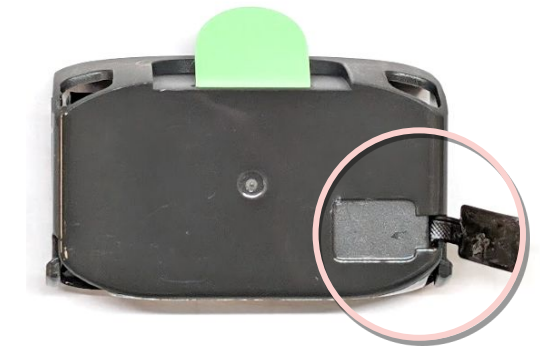
The FPC falls off the battery holder
