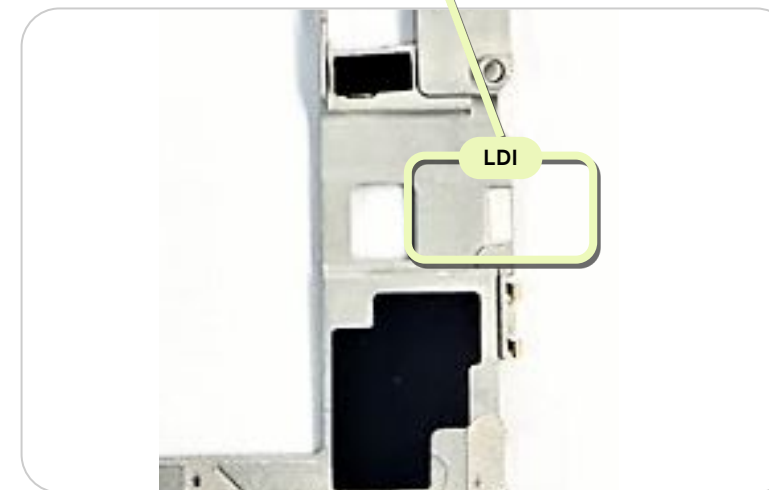
In the SIM card tray slot (on the Mid-frame) visible without disassembling the device.
