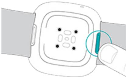
2. To release the latch, slide the flat button toward the band.
