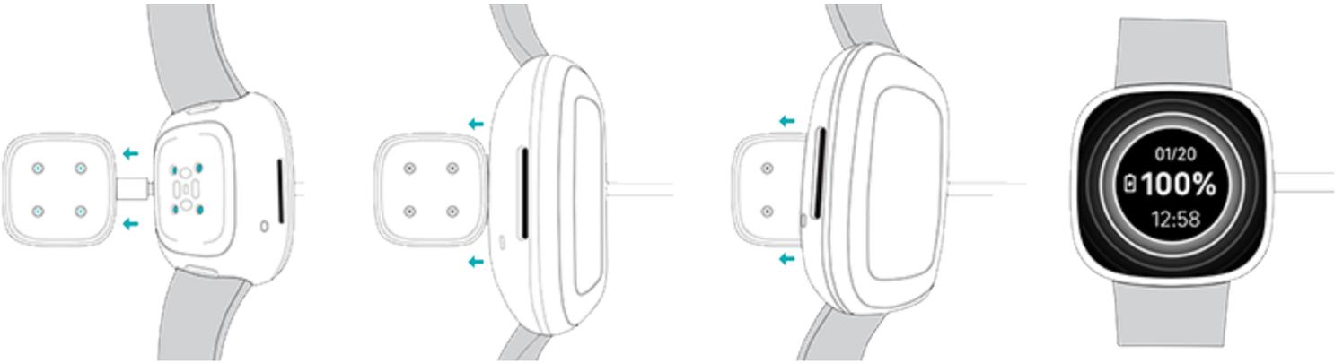
Charge Versa 3 for 12 minutes for 24 hours of battery life. While the watch charges, tap the screen twice or press the button to turn the screen on. The battery level appears for several seconds, then disappears so you can use your watch while it charges. Charging fully takes about 1-2 hours.
