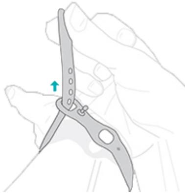
3. Tighten the band until it fits comfortably, and press the peg through one of the holes in the band.
